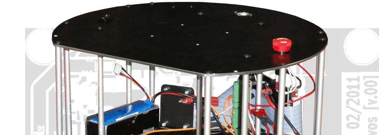
One DC Brushless motor with encoder feedback Two DC motors with encoders feedback Eight digital inputs with adaptive threshold Eight powerful digital outputs open collector INPUT • Eight analog inputs using a A/D with 8 channel and a serial SPI to the FPGA
