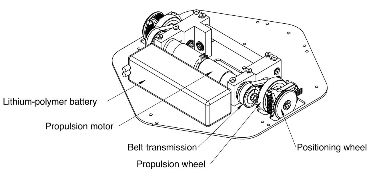
Positioning of the robot is done using dead reckoning. For this we rely on two POSIC quadrature encoders, giving us a resolution of 160 steps per millimeter. To avoid loss of precision due to slippage, those are mounted on separate set of wheels.
