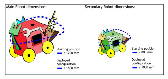
The perimeter of the Main Robot should not exceed 1200 mm at the time of departure. The perimeter of the Main Robot fully extended must not exceed 1600 mm during the match.
